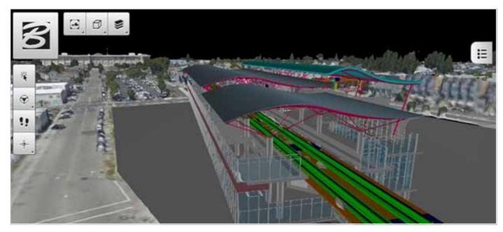
With Navigator Web, any version of an iModel (at any point along its timeline) is accessible in a web browser. This example shows an iModel that aggregates data from Revit, OpenRoads, and AECOsim Building Designer, along with reality context from ContextShare.
