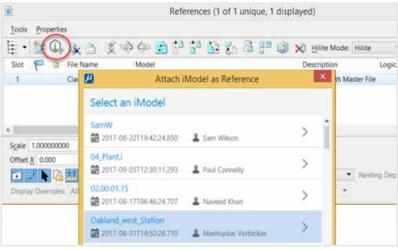
MicroStation CONNECT Edition referencing a physical model from an iModel
