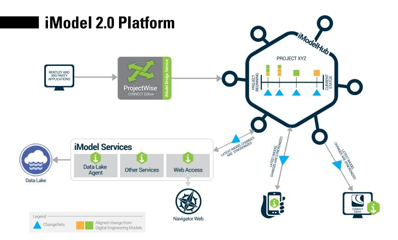
The source of information for the iModel's timeline of changes is ProjectWise workflows; iModel Services and web, mobile, and desktop applications consume iModels.
